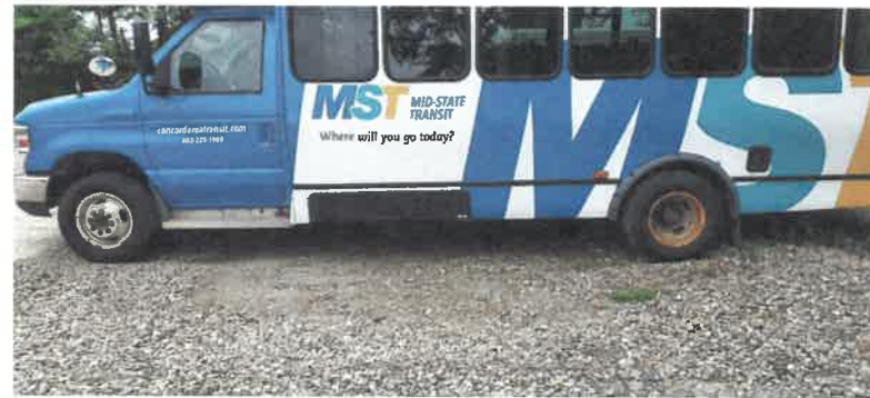
CAPBM: Corrosion on wheels and running board
