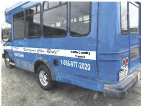
TCCAP: corrosion on body/undercarriage
