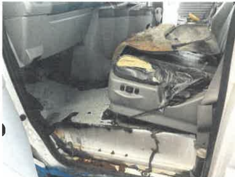
TCCAP: Damage to driver's seat
