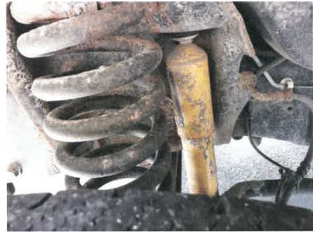
SCS: Undercarriage corrosion
