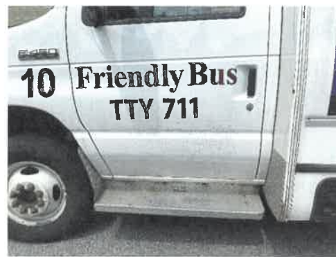
VNA@HCS: Corrosion on running board
